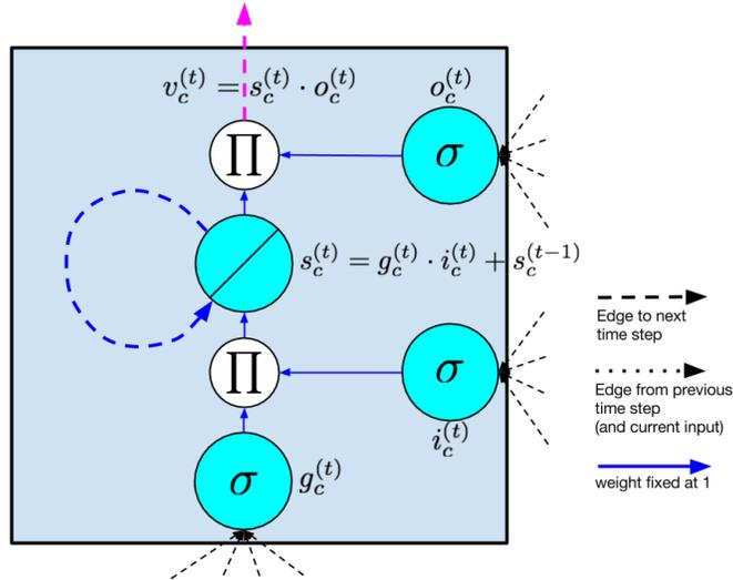
Figure 9: One LSTM memory cell as proposed by Hochreiter and Schmidhuber [1997]. The self-connected node is the internal state  $s$ . The diagonal line indicates that it is linear, i.e. the identity link function is applied. The blue dashed line is the recurrent edge, which has fixed unit weight. Nodes marked  $\Pi$  output the product of their inputs. All edges into and from  $\Pi$  nodes also have fixed unit weight.
