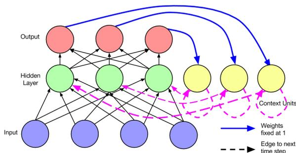
Figure 5: A recurrent neural network as proposed by Jordan [1986]. Output units are connected to special units that at the next time step feed into themselves and into hidden units.
