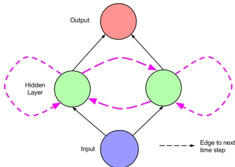
Figure 3: A simple recurrent network. At each time step  $t$ , activation is passed along solid edges as in a feedforward network. Dashed edges connect a source node at each time  $t$  to a target node at each following time  $t + 1$ .
